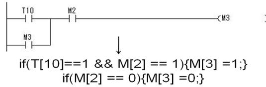
Figure 6: Procedure of LLD convert into VRML
