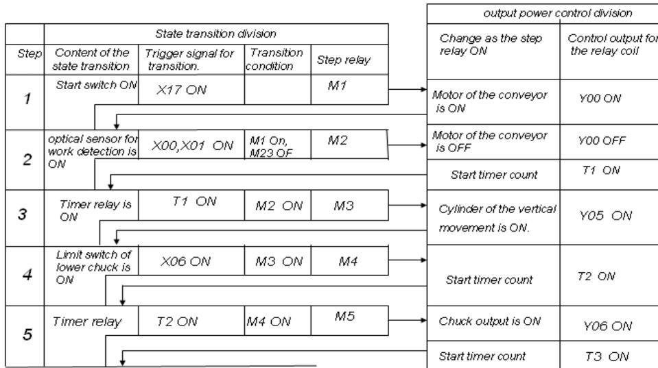
Figure 4: State transition diagram
